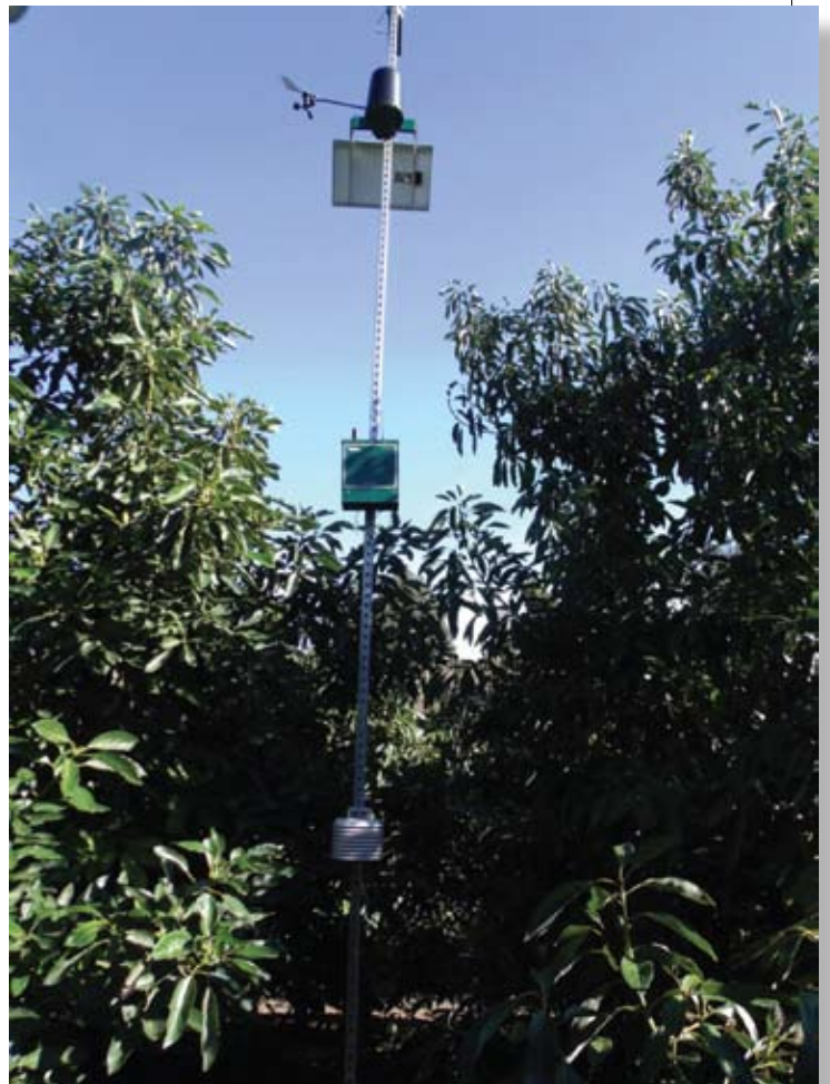
A base station determines ET by tracking variables like temperature, humidity, wind speed, wind direction and rain.
