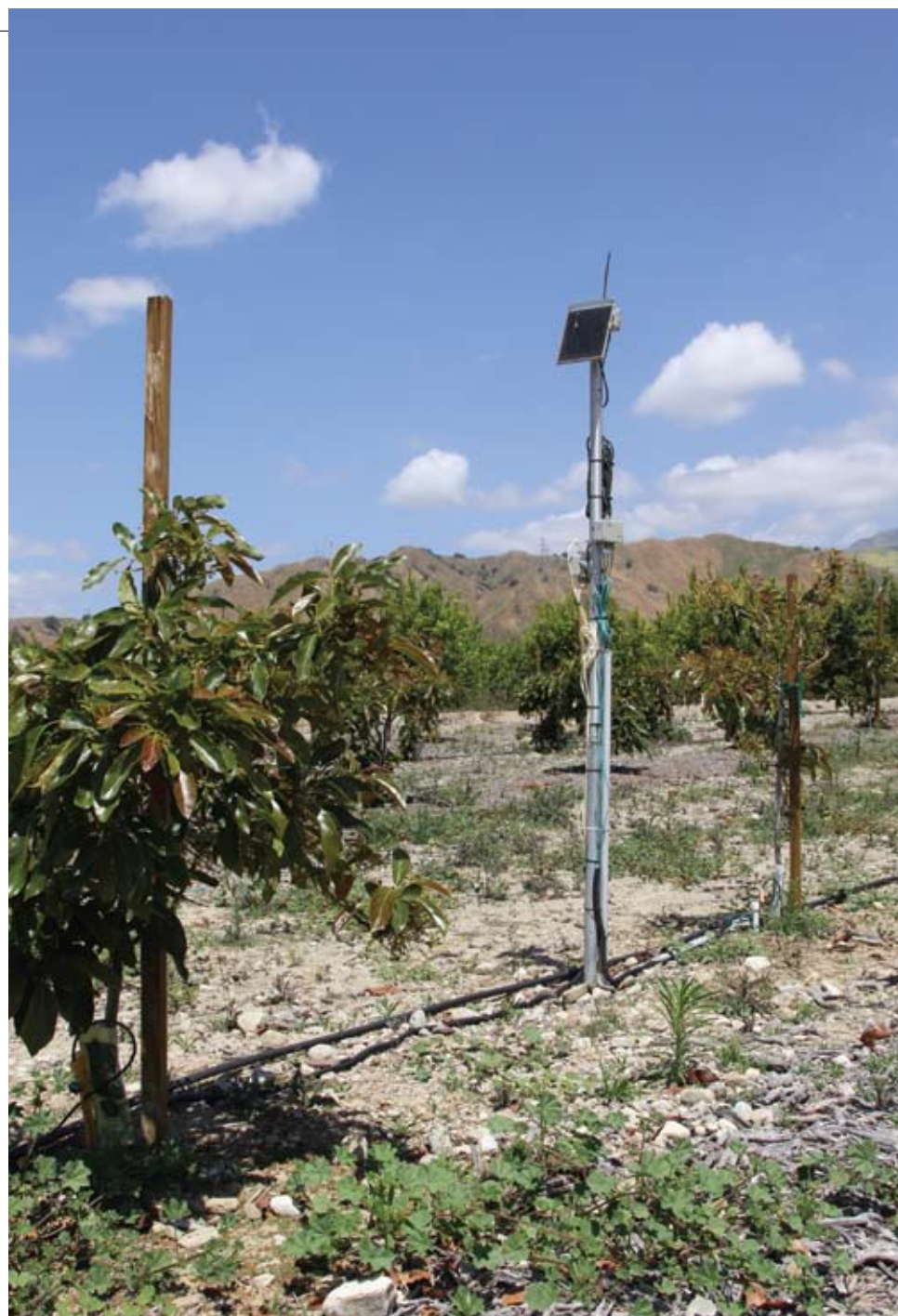
An in-field data logger and radio station used to record and transmit soil moisture sensor data back to the base station.
