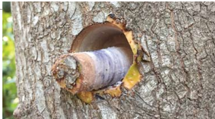
Harvesting a trunk core sample one month after trunk infusion treatments for laboratory bioassays to test chemical efficacy. (Photo courtesy of Dr. Akif Eskalen, UC Riverside)
