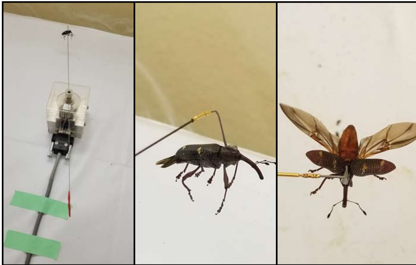
(A) Adult female Heilipus lauri attached to flight mill. (B) Close up of female weevil attached to the flight mill harness which tethers the weevil to the rotor arm of the flight mill. (C) Adult male weevil attached to the flight mill harness with elytra and wings spread in preparation for flight. When weevils commence flight they fly in circles around the pivot point. A lap top computer records distances flown, flight velocity, and periodicity of flight. These flight data can be compared between male and female weevils, young vs. old weevils, virgin vs. mated weevils.
