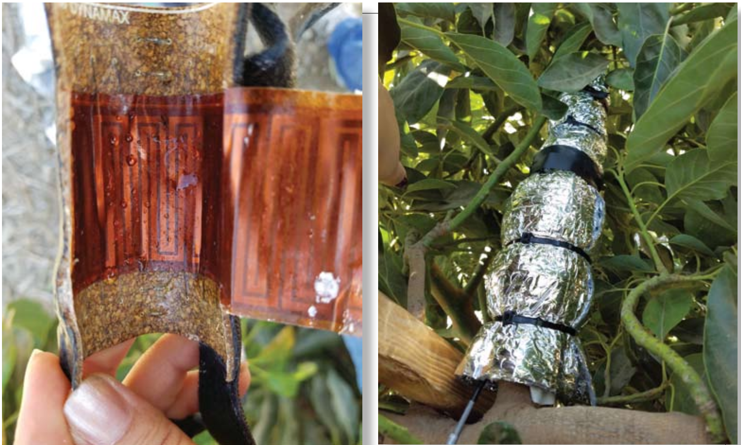
Figure 2. A Dynamax sap flow sensor prior to installation (left) and a sap flow sensor installed on an avocado branch (right). The sensors are installed on branches of about one inch diameter and must be adjusted about every four weeks to account for branch diameter growth. The sensors are hardwired to a base station, which then transmits the data to the internet via a wi-fi connection or cellular modem.
