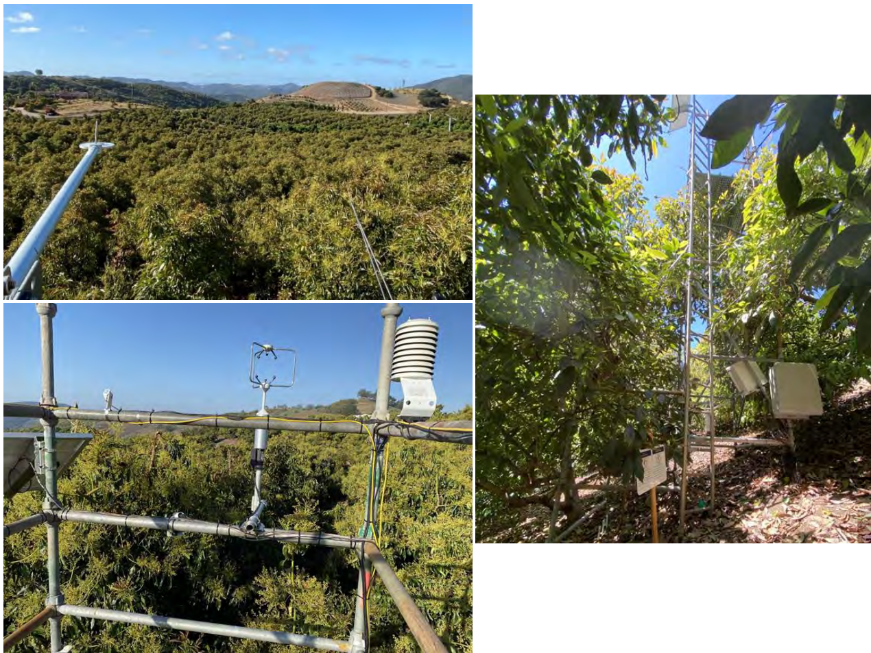
Fig. 1. Ground view of a flux tower/monitoring station in an avocado orchard in Escondido (right). A near look from the top of flux tower demonstrates net radiometer sensor and two fine thermocouple sensors (left up) and sonic anemometer, spectral reflectance sensors, infrared thermometers, and air temperature and relative humidity sensors (left bottom) in an avocado orchard in Temecula.
