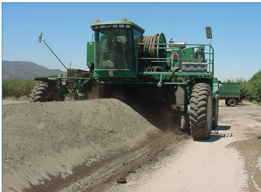
Compost-turning equipment at Groverat Grover Compost in the San Joaquin Valley, California. Compost must maintain a temperature between 131°F ( 55°C) and 170°F for 15 days and be turned a minimum of five times in that 15 day period for a windrow system. Photo: Rex Dufour, NCAT
