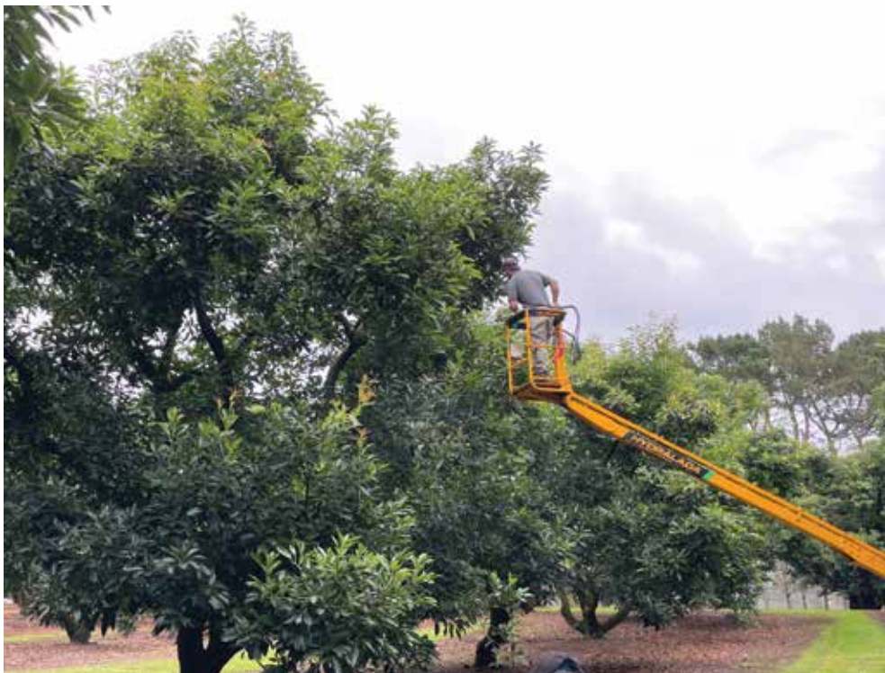
A demonstration of the Hydralada lift platform used for pruning. The Hydraladas used by Maria and Andrew have a maximum height of 8 meters (26 feet).
