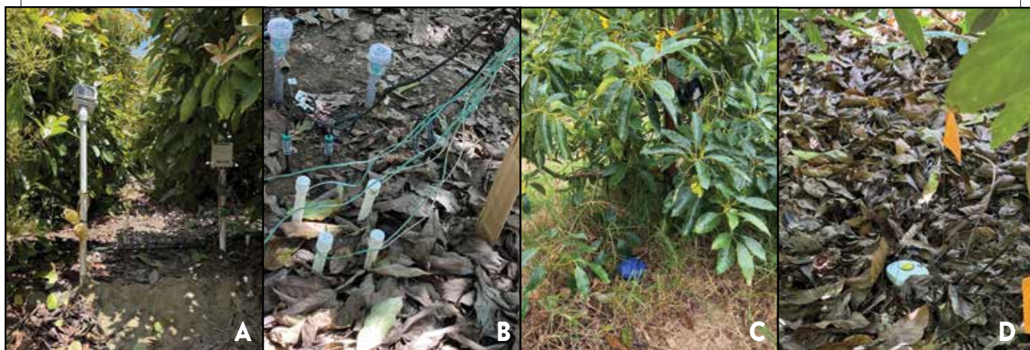
Fig. 3. Various soil moisture sensors used in California avocado orchards (Acclima, Watermark, and tensiometer soil moisture sensors and telemetry devices (a & b), CropX soil moisture probe (c), and Metergroup Teros 54 soil moisture probe (d)).
